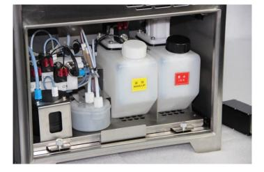
Manual testing: direct manipulation of individual ink system valves and pumps close through the menu, easier to judge the failure, then prevent unnecessary maintenance costs.
