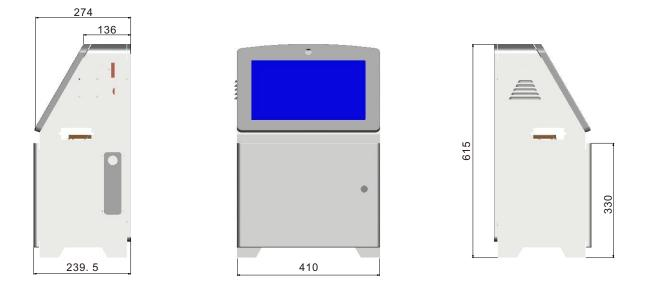
The compact and small design makes it easy to apply to any production line. The aluminum alloy shell can fully protect the machine from damage. The large touch screen design and the internal intelligent system make it easy to edit and print content.
